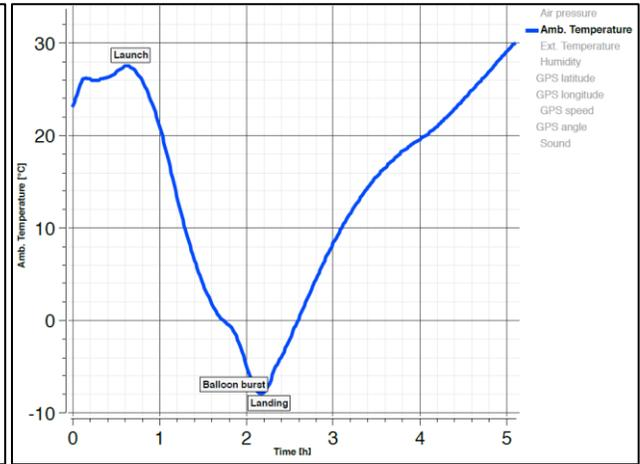
Temperature Inside the Payload
