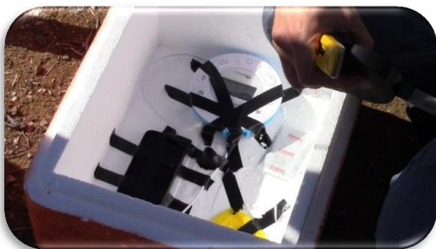
Include a Labdisc GenSci or Labdisc Enviro as part of the payload of a high-altitude near-space weather balloon to record temperature, air pressure, sound and GPS location during the high-altitude weather balloons ascent and descent. Additional equipment in the payload could include a HD video camera and GPS tracking unit to ensure that you recover the balloon's payload.
