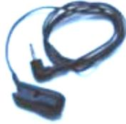
3. Connect the ear-clip
