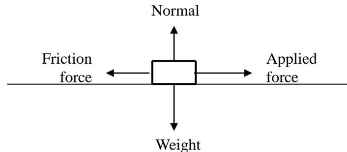
**Friction can be static or kinetic.** Kinetic happens when a body is moving, that is, its speed is nonzero. By contrast, static friction occurs when the velocity of a body is zero.
