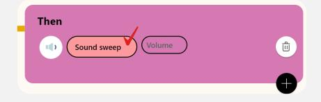
Next, in the "Condition" key, we select the "Sound sweep" option. This option will generate all 16 Xploris tones when the Distance sensor is between the 30-300cm range.
