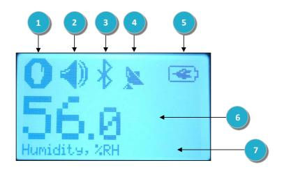
① Run/Stop icon – shows when the Labdisc is logging data, or when the Labdisc is not logging sensor data.
