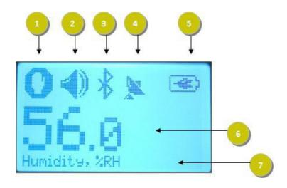
① Run/Stop icon – shows when the Labdisc is logging data, or when the Labdisc is not logging sensor data.
