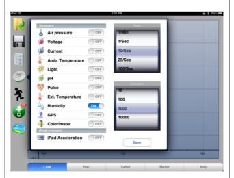
Just click on the **RUN** icon and relative humidity measurement stream will build as a line graph on the iPad.
