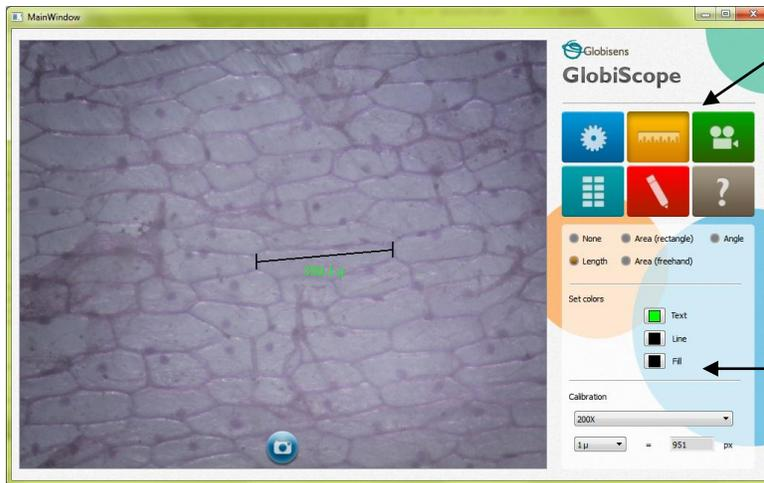
To the right of the main display screen **six icon buttons** control all the GlobiScope features: Settings, Measurements, Movie capture, Gallery, Graphics, Annotation and Help.
