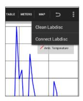
You cannot clear the Labdisc memory directly from the Labdisc. You must be connected to a computer, iPad or tablet.
