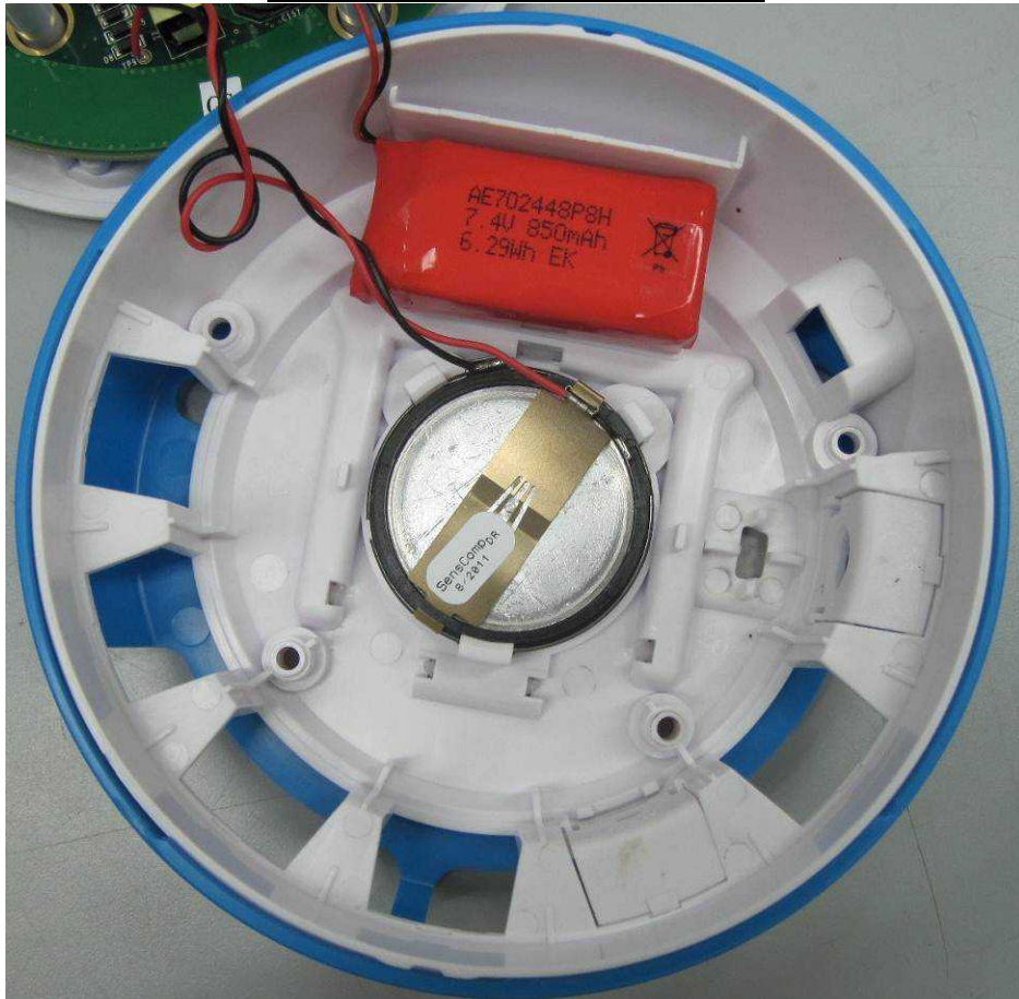
Photo #13 - Bottom cover internal view
