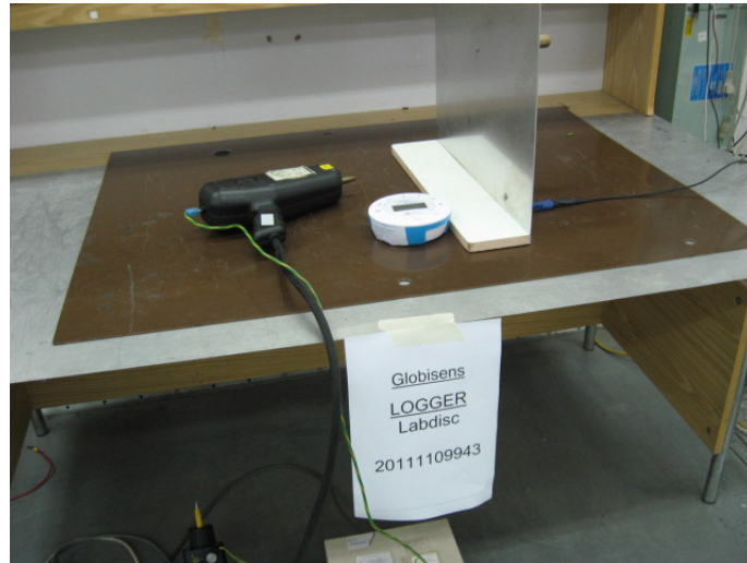
Figure 9. Immunity to Electrostatic Discharge Test
